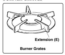
The grates are porcelain enameled cast iron or steel. They should be washed regularly and especially after spillovers. When replacing grates on the burner plates (C), the extension (E) is indexed into indentation (E) directly across from the igniter (D). See illustration Page 22, under Burner Plates.
